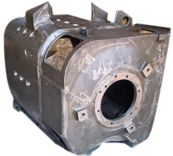
Magnetic frame used in Locomotives supplied to GE Transportation, Erie, Pennsylvania. Main body hot-formed from 60 mm thick plate.
